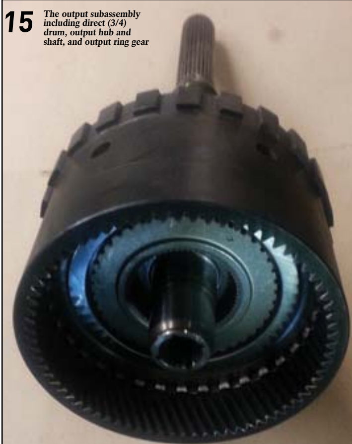
The AOD/AODE/4R70W family of transmission use a single "Ravigneaux" planetary gearset. This unique planetary gear design is unique with one carrier that has a long and short set of pinions, two sun gears and a single output ring gear. Most overdrive type automatic transmissions have 3 planetary gearsets. It is this geartrain that allows the LenTech Reverse/Third modified powerflow to bolster third gear torque capacity
