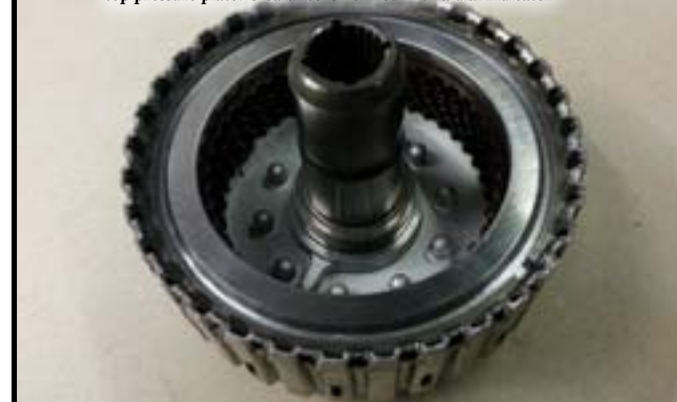
10 The completed 3rd/4th (direct) drum. The extra friction capacity is achieved with thinner steels and machining of the piston and top pressure plate. Clearance is verified with a dial indicator
