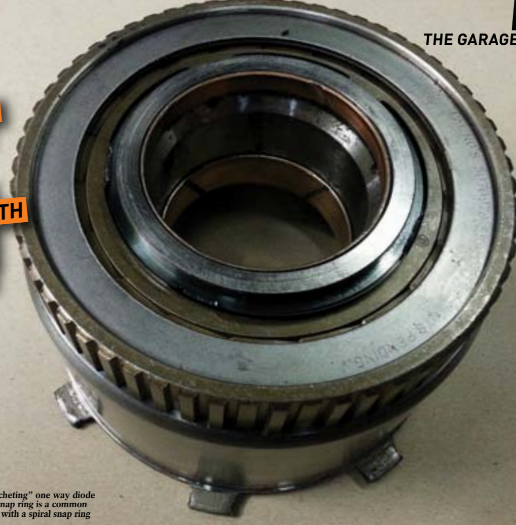
9 FWD input drum with original lockup type input shaft pressed in, and the intermediate "stub" shaft which splines to the FWD and direct drums. On the right, the billet 1pc nonlock input shaft for comparison. Top left, thick cushion wave plate and OE paper friction. Bottom left, Thinner cushion wave plate and Exedy friction
