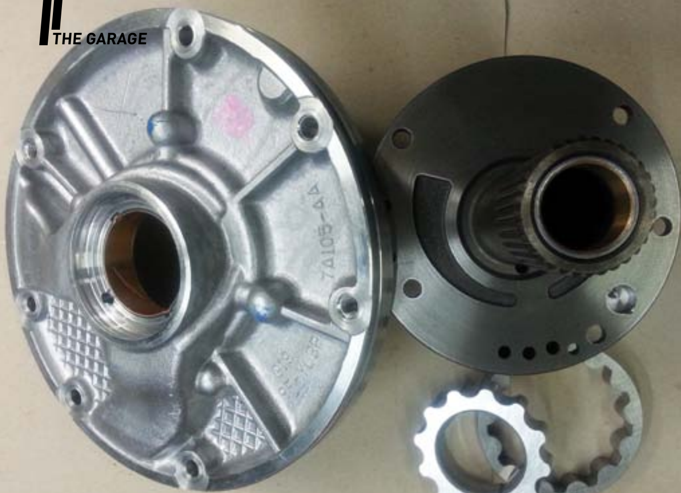
12 This photo shows the Strip Terminator AODE/4R70W oil pump. The original OE pump body is aluminium. As this model has eliminated lockup and is fitted with a billet 1 piece input shaft, a modified AOD pump stator support is used. This gerotor pump has good volume and pressure and has proven reliable
