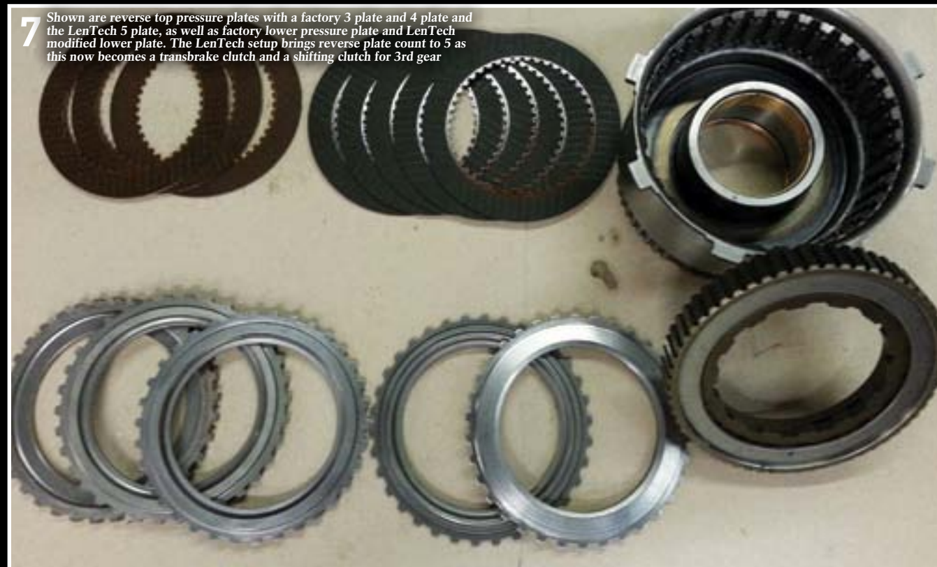
6 Early AODE/4R70 transmission models were built with paper frictions and while V8 vehicles got 6 frictions, 6 cylinders got 5. This Strip Terminator has no fewer than 8 frictions
