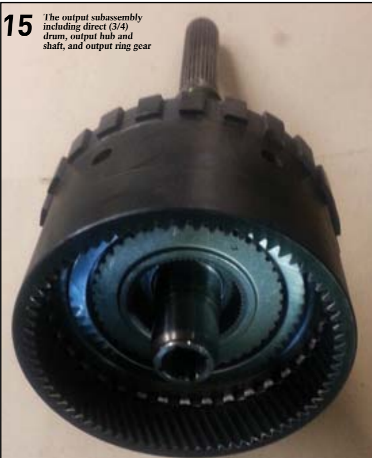
The AOD/AODE/4R70W family of transmission use a single "Ravigneaux" planetary gearset. This unique planetary gear design is unique with one carrier that has a long and short set of pinions, two sun gears and a single output ring gear. Most overdrive type automatic transmissions have 3 planetary gearsets. It is this geartrain that allows the LenTech Reverse/Third modified powerflow to bolster third gear torque capacity
