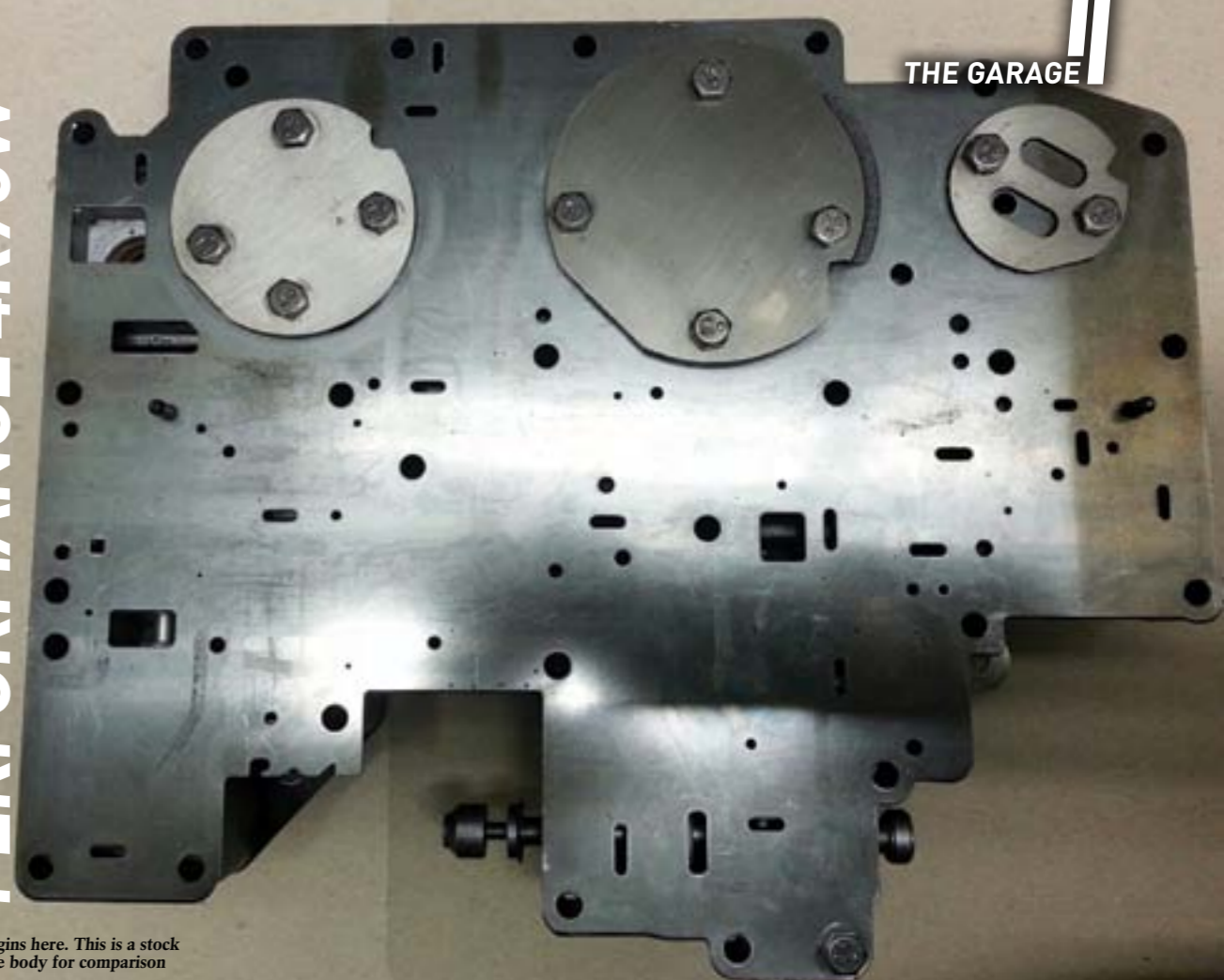
2 Here is the machined area to accept the transbrake solenoid
