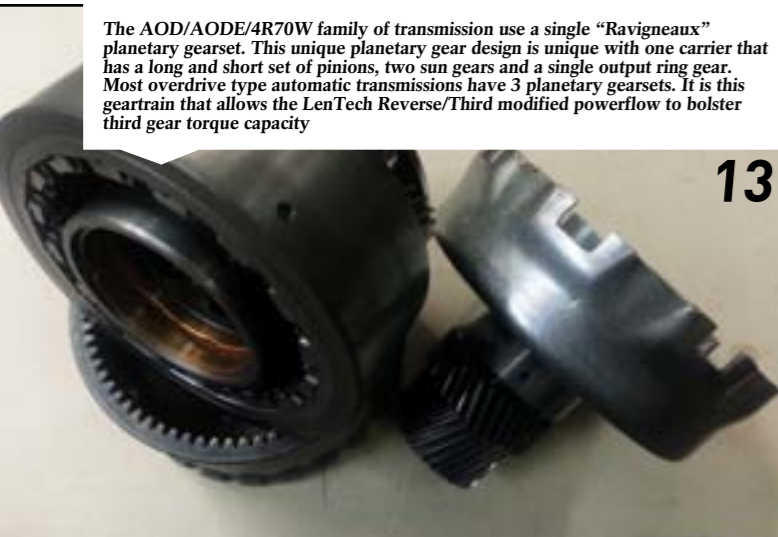
14 A look into the planet carrier reveals the long and short set of pinions
